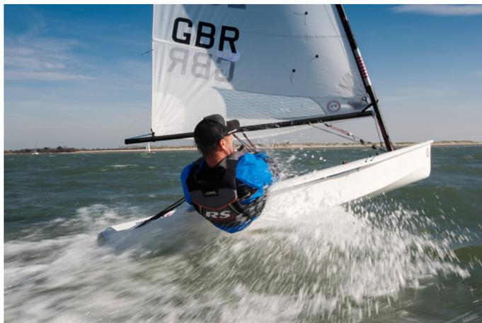
The company found through testing that a 4 m long hull would be long enough to support the larger helmsman, without being too much of a handful for small sailors to launch and recover.
